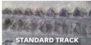
After 180 hours of aggressive testing, the standard track failed, while the Camso track continued for 20 hours more. Which means that Camso track provides at least 10% more life.
