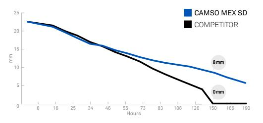
In this test, we clearly see that the competitor track tread compound was wearing faster versus Camso. Maintaining more rubber around the carcass offers more protection and translates in longer service life.
